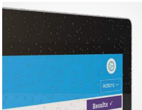
Moisture resistant medical-grade front panel
